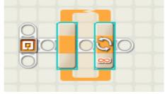
With the loop command highlighted, verify the loop control is set to forever in the control panel.
