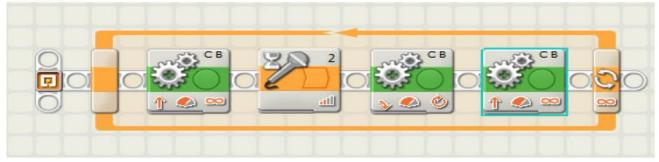
With the move command highlighted, verify the following settings in the control panel.
