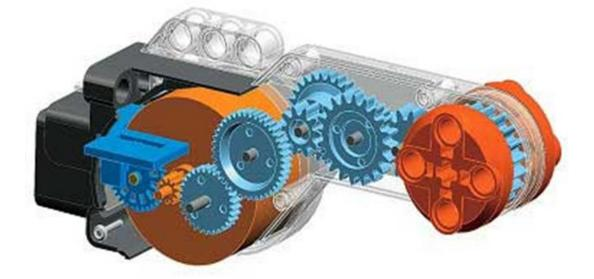
For example, a gear ratio of 10:1 is 10 rotations of a small gear resulting in 1 rotation of a big gear, although some imperfection in the meshing of gears reduces the precision of rotations (+/- 1 degree accuracy)
