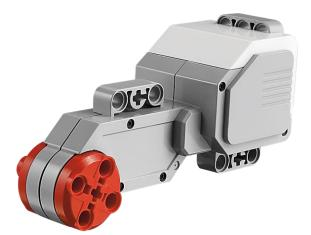
This motor has lots of gears within it, which explains its size and shape.
