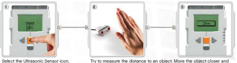
Select the Ultrasonic Sensor icon. Select the port in which you have placed the sensor.
