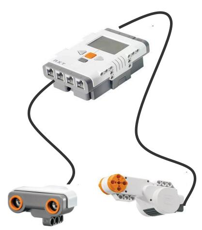
Do This: Connect the LEGO brick to the ultrasonic sensor and a motor, as shown to the left.
