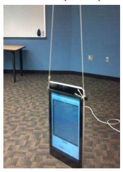
Example 1. Cable ties hold a 7-inch tablet. The ties were tight enough to hold the tablet in place, but could be removed and reattached. Unseen in this photograph, the strings were tied directly to a ceiling girder.
