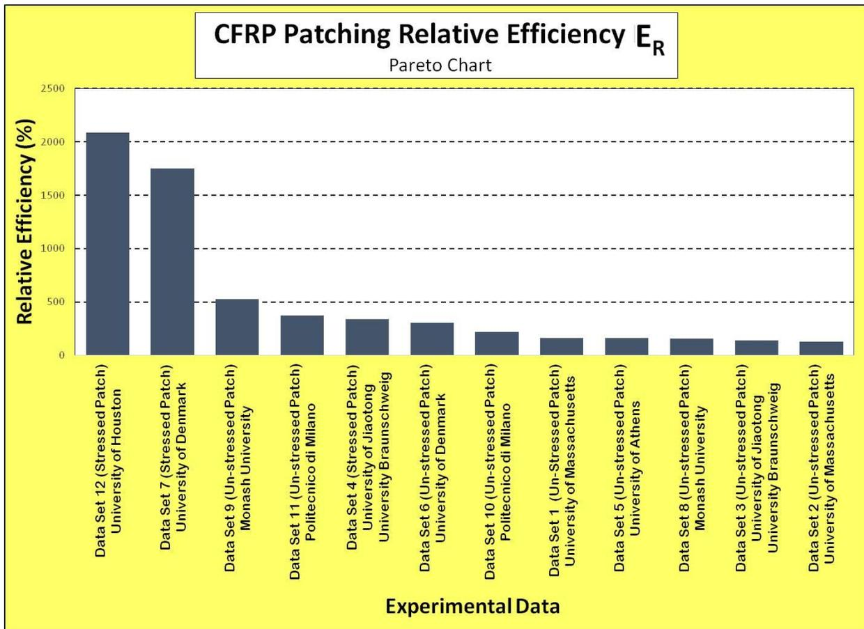
**Figure N.** *CFRP Relative Efficiencies Pareto Chart.* In this Pareto chart, it can be seen that the repair methods using pre-stressed CFRP patches are among the first five most-efficient procedures.
