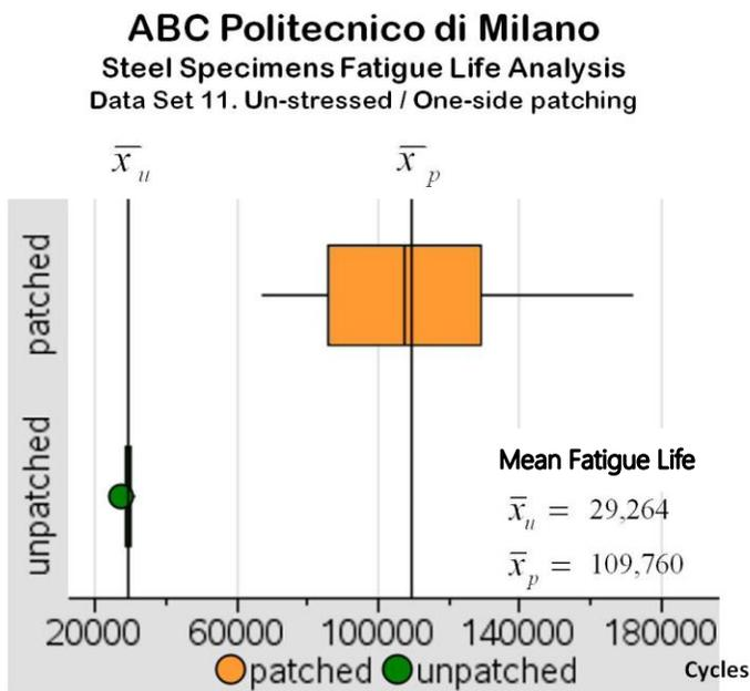
**Figure K.** The second repair method proposed by the ABC Politecnico di Milano is expected to increase the mean fatigue life of cracked steel specimens about 3.75 times and be effective 100% of the time.
