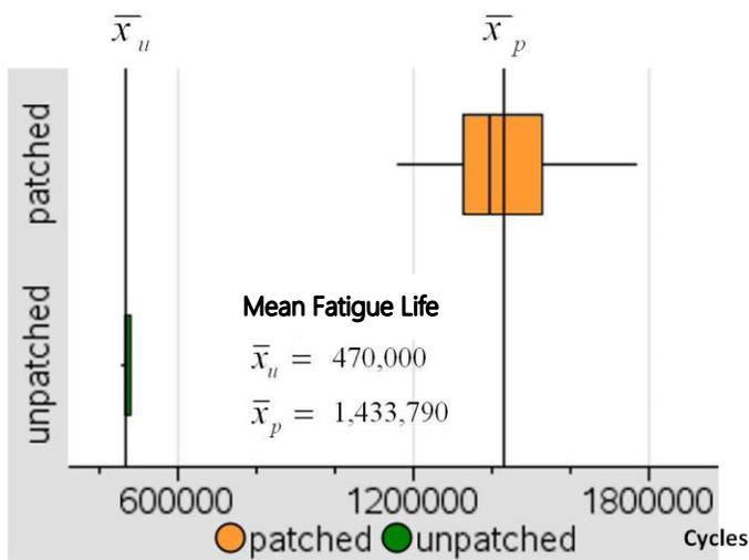
**Figure F.** The first repair method proposed by the Technical University of Denmark is expected to increase the mean fatigue life of cracked steel specimens about 3 times and be effective 100% of the time.
