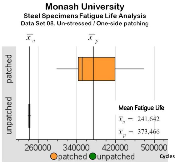
**Figure H.** The first repair method proposed by Monash University is expected to increase the mean fatigue life of cracked steel specimens about 1.5 times and be effective 100% of the time. This box-and-whisker plot compares the fatigue life data of patched and unpatched specimens tested at Monash University.
