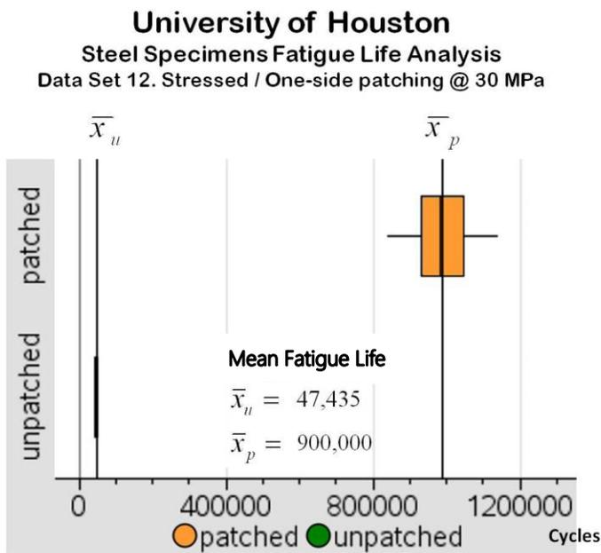
**Figure L.** The repair method proposed by the University of Houston is expected to increase the mean fatigue life of cracked steel specimens about 21 times and be effective 100% of the time.
