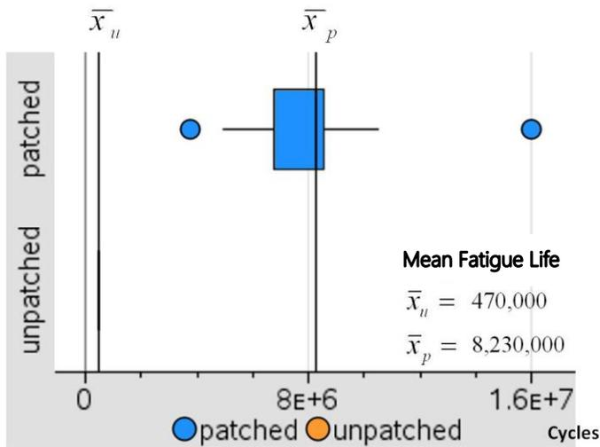
**Figure G.** The second repair method proposed by the Technical University of Denmark is expected to increase the mean fatigue life of cracked steel specimens about 17.5 times and be effective 100% of the time.
