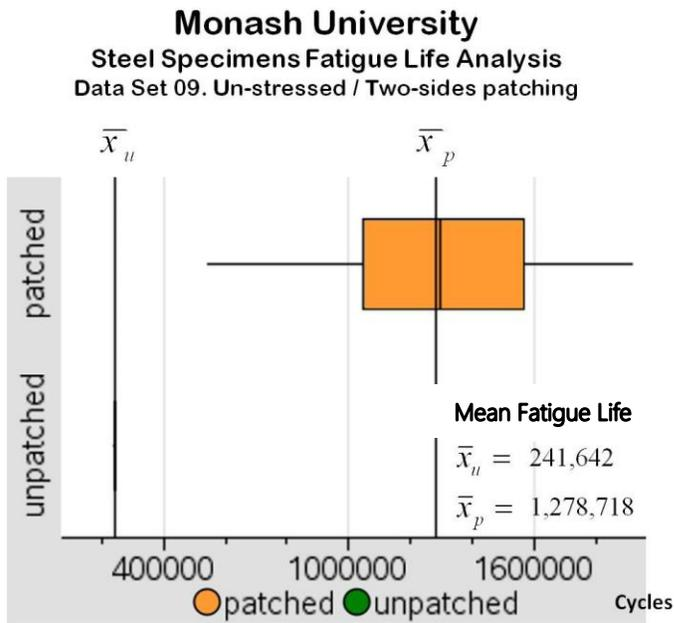
**Figure I.** The second repair method proposed by Monash University is expected to increase the mean fatigue life of cracked steel specimens about 5.3 times and be effective 100% of the time. This box-and-whisker plot compares the fatigue life data of patched and unpatched specimens tested at Monash University.
