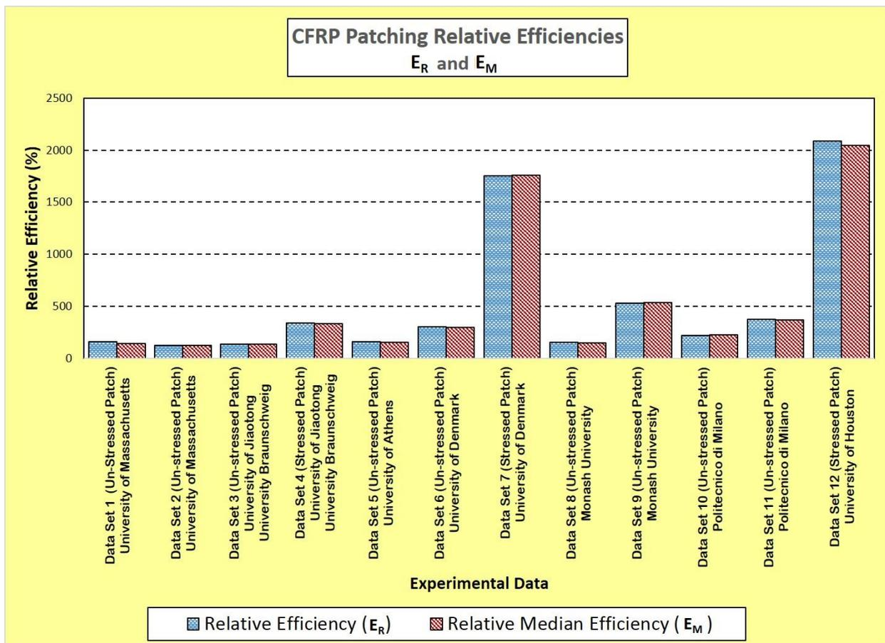
**Figure M.** CFRP Relative Efficiencies Graphical Comparison.
