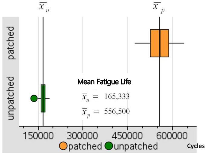
**Figure D.** The second repair method proposed by the Universities of Jiatong and Braunschweig is expected to increase the mean fatigue life of cracked steel specimens about 3.4 times and be effective 100% of the time. This box-and-whisker plot compares the fatigue life data of patched and unpatched specimens, tested at the Universities of Jiatong and Braunschweig.
