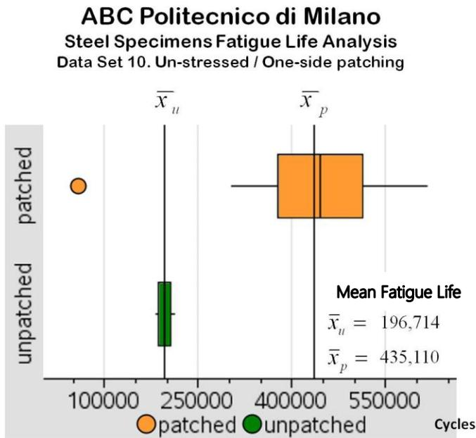
**Figure J.** The first repair method proposed by the ABC Politecnico di Milano is expected to increase the mean fatigue life of cracked steel specimens about 2.2 times and be effective practically 100% of the time.
