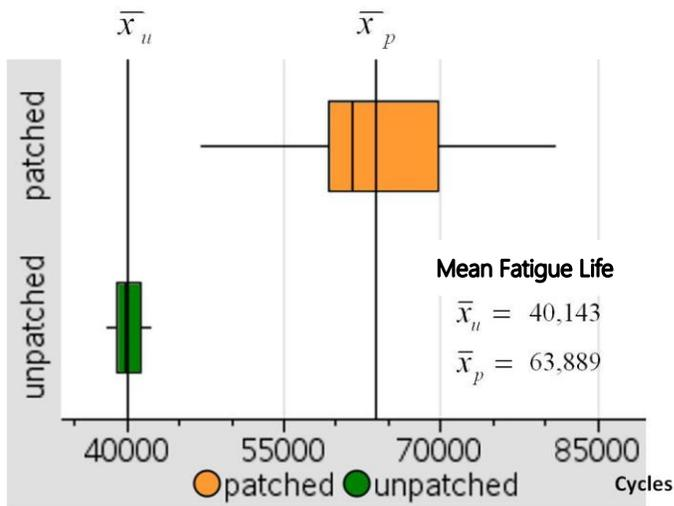
**Figure E.** The repair method proposed by the National Technical University of Athens is expected to increase the mean fatigue life of cracked steel specimens about 1.6 times and be effective 100% of the time.
