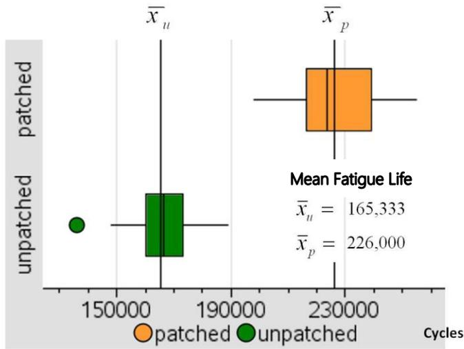
**Figure C.** The first repair method proposed by the Universities of Jiatong and Braunschweig is expected to increase the mean fatigue life of cracked steel specimens about 1.4 times and be effective 100% of the time.
