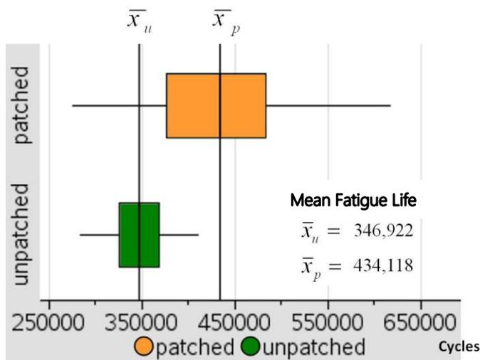
**Figure B.** The second repair method proposed by the University of Massachusetts is expected to increase the mean fatigue life of cracked steel specimens about 1.25 times and be effective about 50% of the time.
