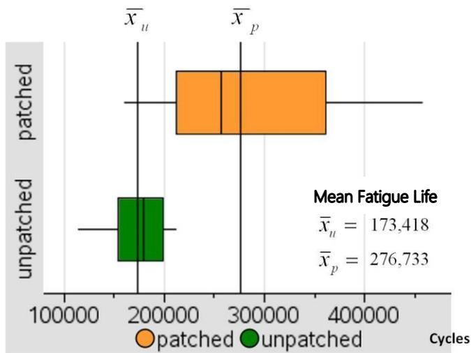
**Figure A.** The first repair method proposed by the University of Massachusetts is expected to increase the mean fatigue life of cracked steel specimens about 1.6 times and be effective about 75% of the time.
