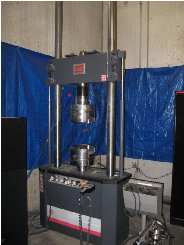
Figure 1. A servo hydraulic test system is used to apply constant and periodic forces on rigid objects such as steel bars. A connected computer system records the entire process until the tested element fails.
