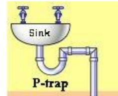
A septic tank naturally produces gases (caused by bacteria breaking down the organic material in the wastewater), and these gases do not smell good. Therefore, sinks have pipe bends called **P-traps** that hold water in the lower loop to block gases from flowing back into the house. The gases flow up a vent pipe instead; notice the roof of any house to see one or more vent pipes poking through.
