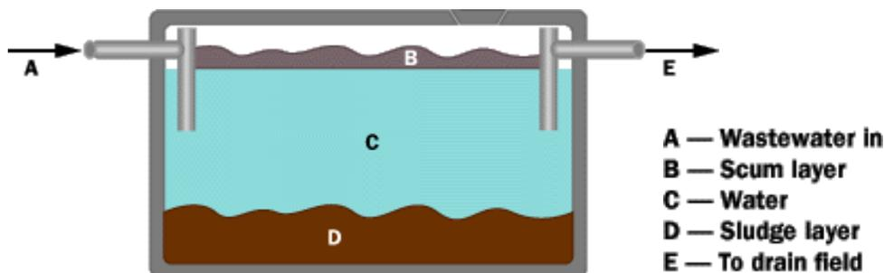
In this side-view drawing of a septic tank, you can see three layers. Anything that floats rises to the top and forms a layer known as the **scum layer**. Anything heavier than water sinks to form the **sludge layer**. In the middle is a fairly clear water layer that contains bacteria and chemicals (such as nitrogen and phosphorous that act as fertilizers), but is largely free of solids.
