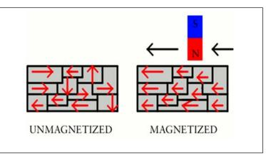
Traditional Bulk Magnetic Material: Figure shows a gradual alignment of domains with direction of magnet as a magnetic field is applied in two dimensions. Three dimensional alignments of domains occur in real materials. KEY: bulk material (polycrystalline) will have numerous domains as indicated above.
