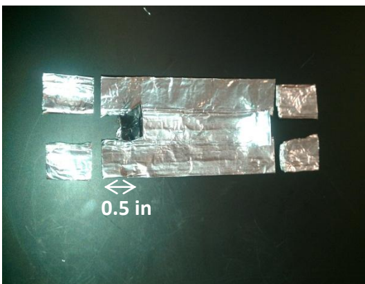
Cut outer tabs down to 0.5-in on both sides
