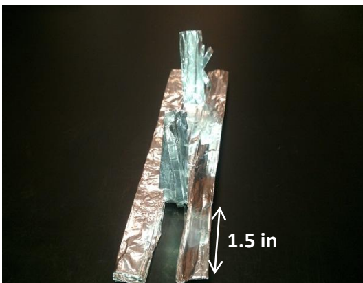
Cut base on both sides of left and right sides 1.5 in in towards center
