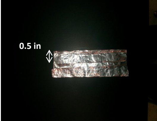
Rotate foil 90 degrees and fold top and bottom edges 0.5-in towards center →
