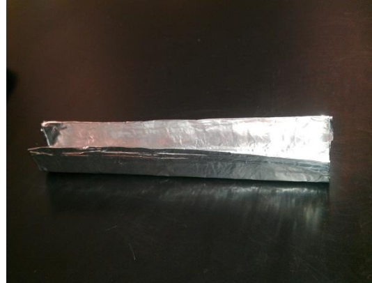
Flip foil over and fold top and bottom sides up forming a U shape with 0.5-in wide base
