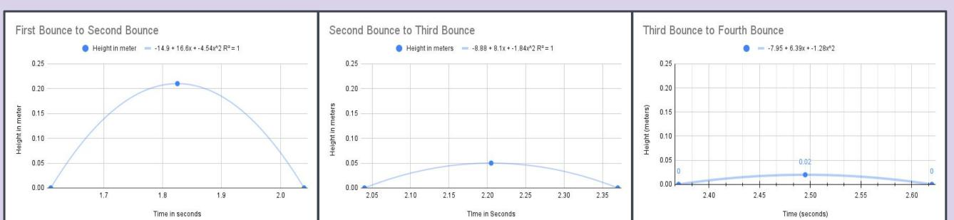
Our goal was to use this research to determine the optimal ball to be used as the score ball in the game. As can be seen from the graphs, the wiffle ball loses a large amount of its energy through its bounce, which makes it a good candidate for our game. Its properties force the players to hit the ball more times to score, keeping the velocity of the score ball low while the velocities of the hitter balls are high.
