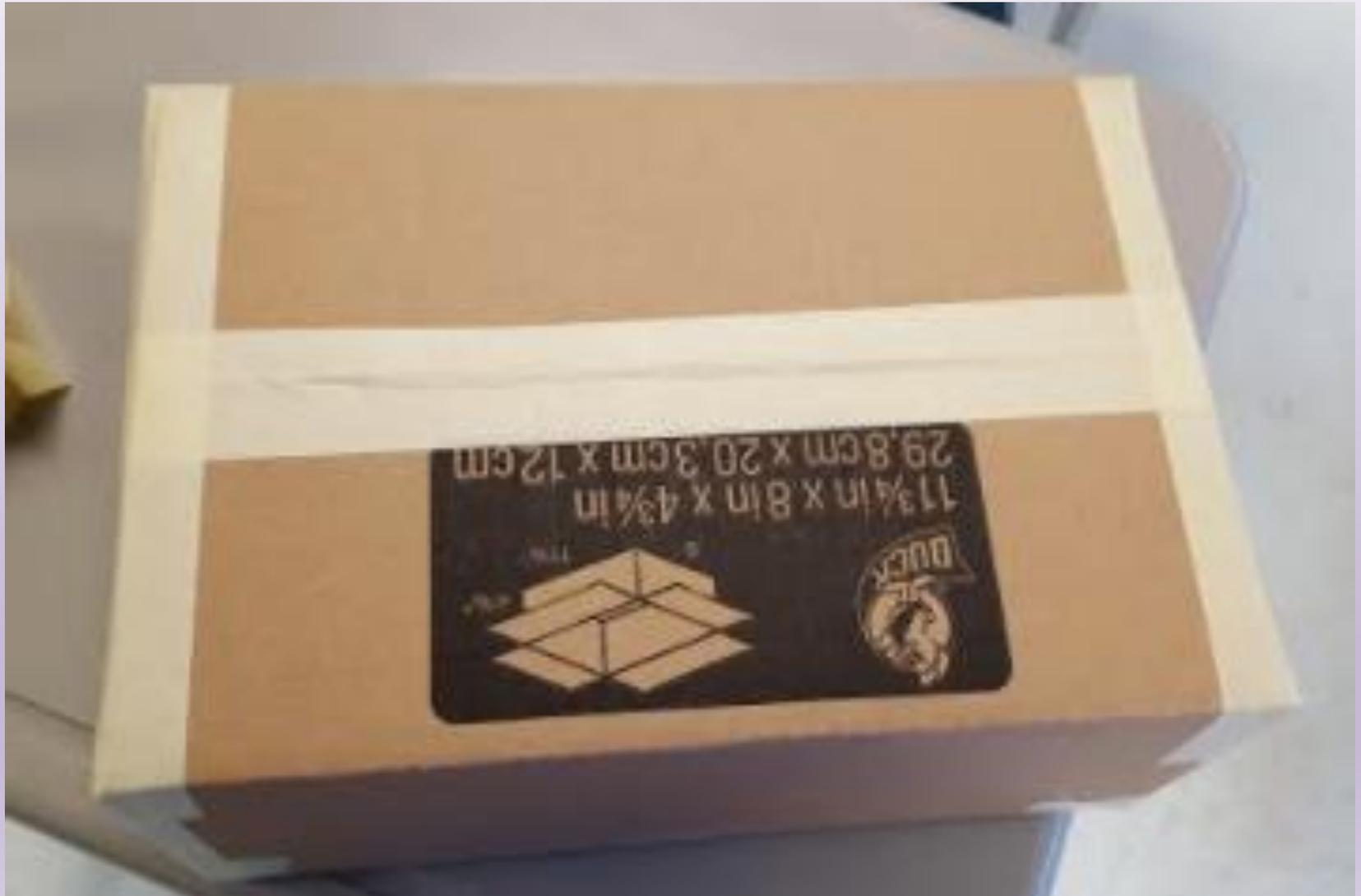
Make sure all the sides are covered with tape to keep out ambient light
