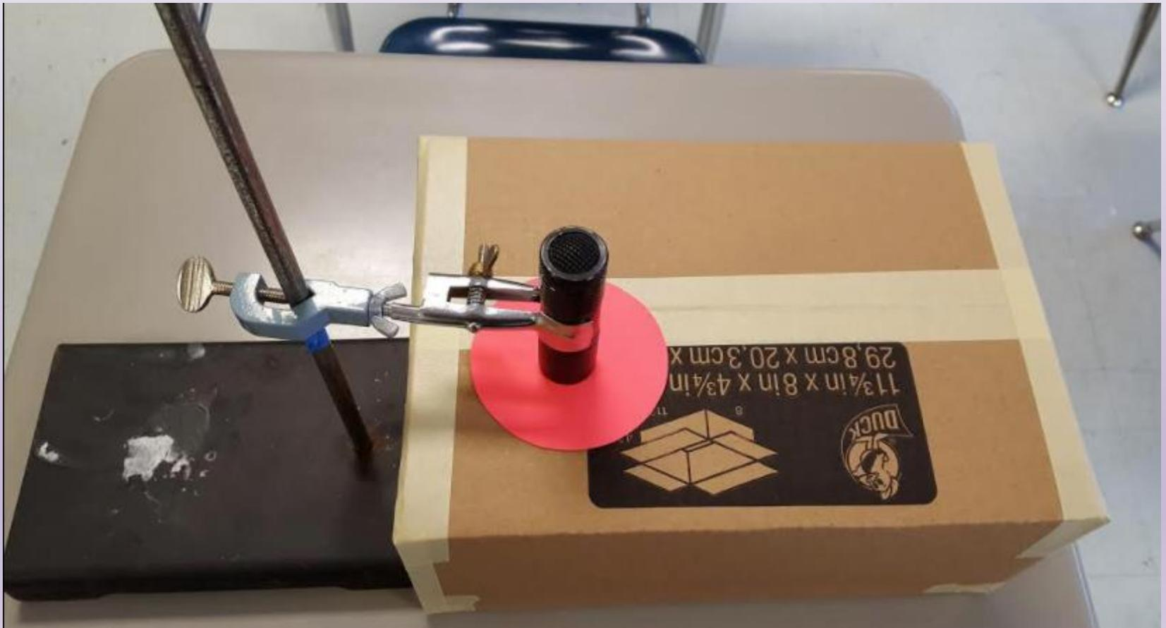
Place the light sensor probe (also secured upright by using a clamp and ring stand) next to the UV flashlight on the round template
