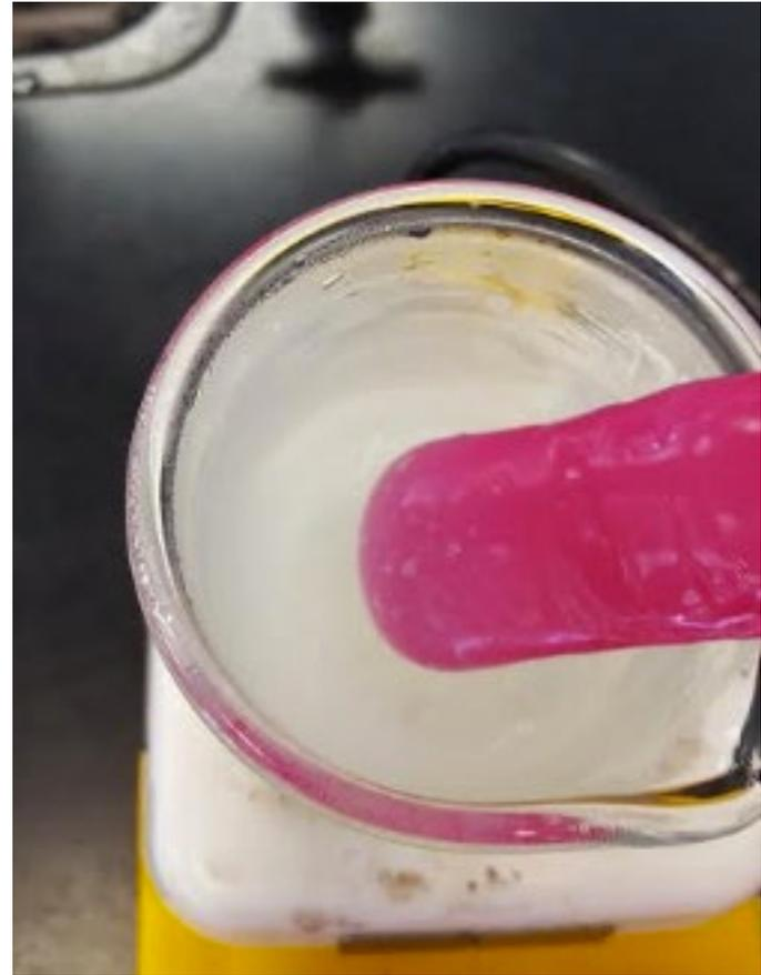
Transfer the heated mixture to a prepared petri dish using the spatula; let sit and dry overnight
