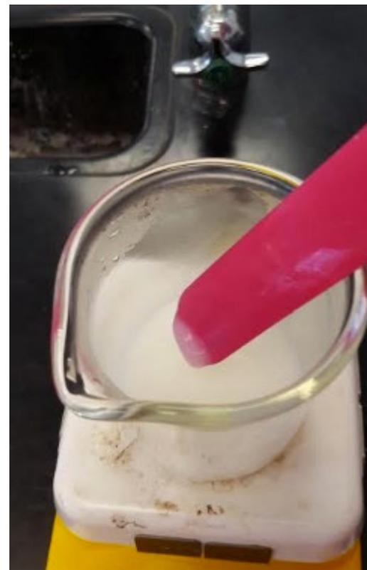
After 6 minutes and 30 seconds, the mixture will become a clear and/or a viscous solid
