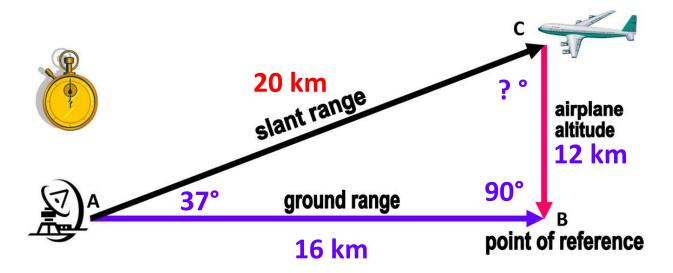
Use your scale to find the ground range and the airplane's altitude in your radar triangle model. Example answers for scale: 1 km = 1 cm
