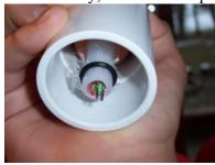
Simply remove the O-ring and cover with a new piece of plastic.
