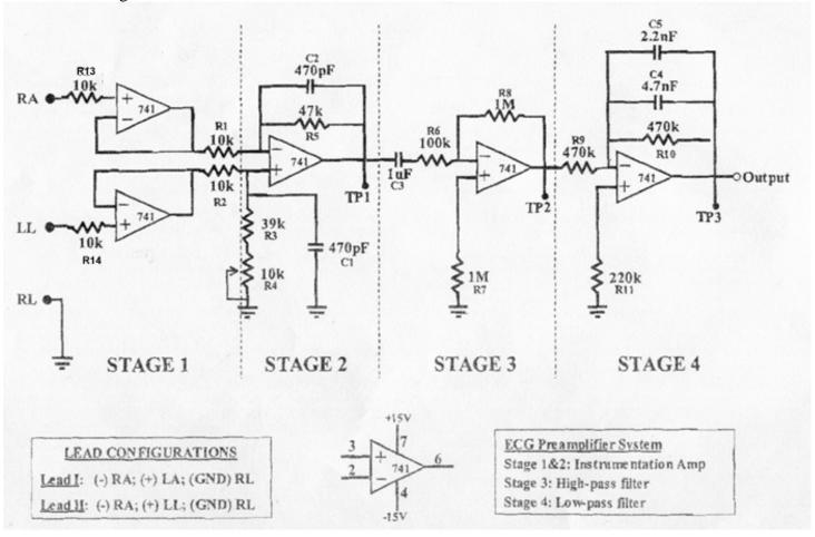
Prepare the circuit on a breadboard, arranging each stage as a separate section. It should look similar to this:
