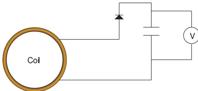
The diode will prevent any induced current in a certain direction, so that there will only be induced current either when the second coil is connected or disconnected to the battery. The voltmeter will read the voltage across the capacitor, giving you a reading of how much charge has been deposited from the induced current.
