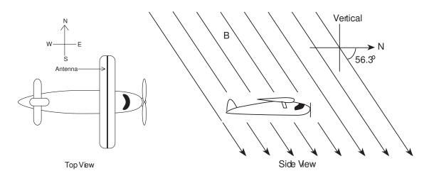
An airplane has a copper antenna attached to its wing that extends 20 m from wingtip to wingtip. The plane is traveling north at 95 m/s in a region where Earth's magnetic field has a vertical component and a northward component. The magnitude of the magnetic field is at an angle of  $56.3^{\circ}$  from the horizontal and has a magnitude of  $6.5 \times 10^{-5}$  T.
