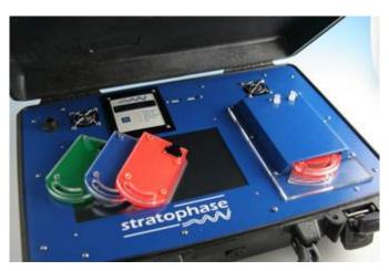
antibodies on the chip result in localized changes in the refractive-index. This increases the wavelength of the reflected light which can be detected. With one chip it is possible to multiplex 16 different biological agents like spores, viruses and toxins in real-time. You can either load samples manually or, when continuous monitoring is necessary, the cartridge can be combined with air sampling technology.
