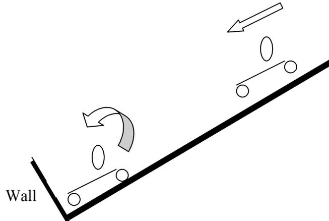
The center of gravity of the car was above the plane of the chassis. So why doesn't the car flip forward at low speeds? As the car rotates, the center of gravity has to rise up, thus requiring potential energy. Therefore, the terminal velocity and its associated kinetic energy need to be sufficient to rotate the center of gravity up and over.
