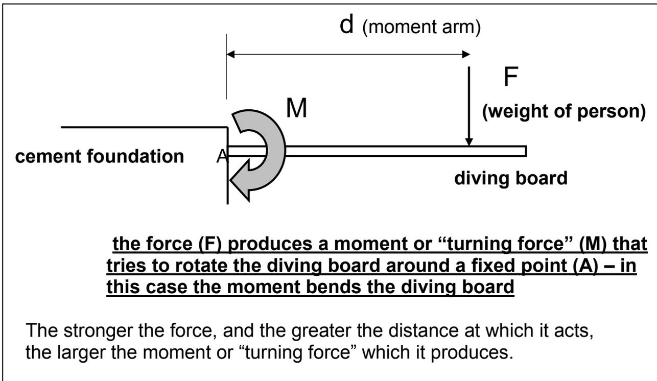
A moment or “turning force” (M) is calculated by multiplying a force (F) by its moment arm (d) – the moment arm is the distance at which the force is applied, taken from the fixed point:
