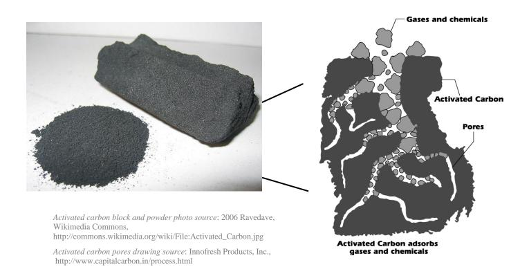
In this lab, we are going to test to see how well Brita® household water filters which use activated carbon, remove chlorine from bleach water. Chlorine is used as a disinfectant in treating drinking water, but too much chlorine in drinking water is dangerous—it damages your nervous system and may cause cancer.
